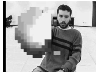
Figure 1: The motion history image represents how recently motion was detected at each pixel location. Pixels currently in motion are shown as white, while pixels in motion in the recent past are shown in decaying shades of gray.
